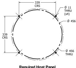
Required Host Panel Fixing Detail
